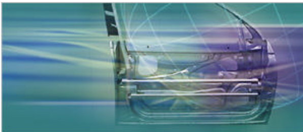
Figure 1: Side impact beams in the complete door frame.
